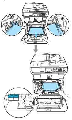
Insert the original orange packing material for locking the belt unit as shown in the illustration.
